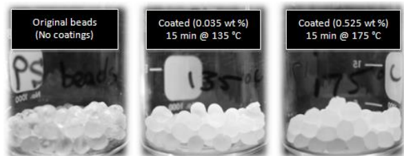
Figure 3: The polystyrene beads before and after being coated with hybrid mesoporous silica powder in the dynamic coating experiments
