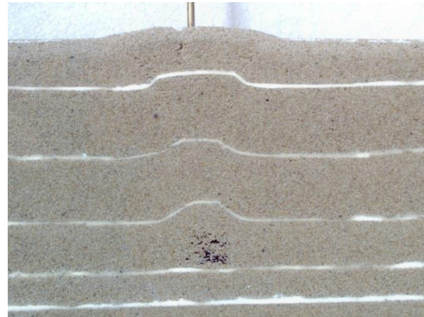
Photo 1 Sand displacement due to horizontal strip anchor uplift
