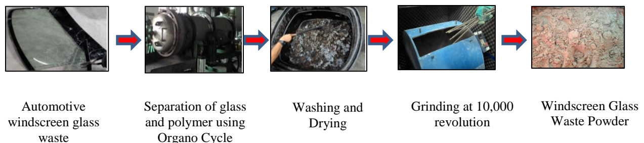
Fig 1 Preparation of automotive windscreen glass waste powder (WGWP)
