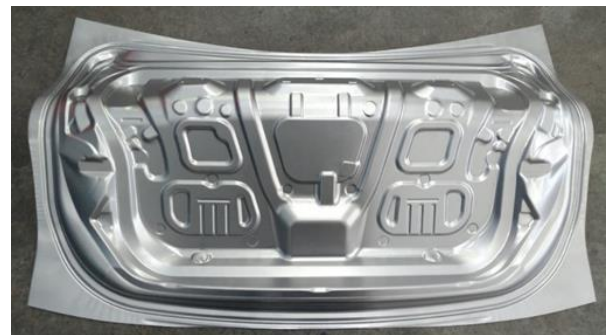
Figure 2.3 Trial product for Trunk Lid panel after yield reduction
