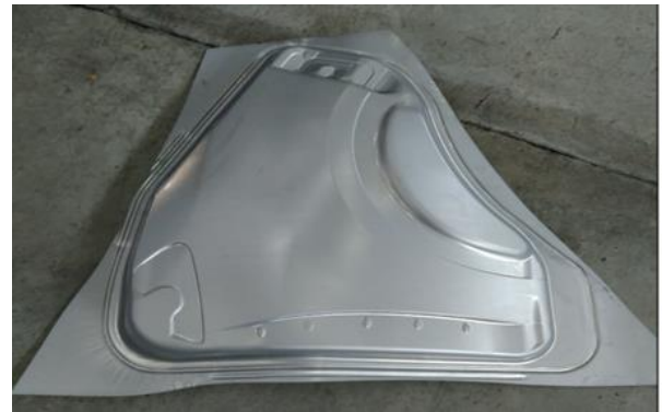
Figure 2.1 Trial product for Front Fender panel after yield reduction
