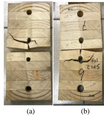
Fig. 6. Typical failure modes of glulam sample due to single shear test for Pine (a) 12 mm diameter and (b) 14 mm diameter
