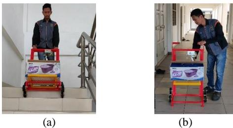
Figure 9: Physical testing of the designed trolley with loads 20kg
