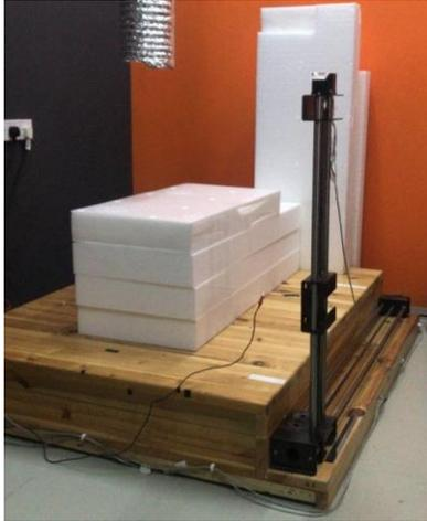
Figure 3 CNC hot wire cutter machine at IFCON (M) Sdn Bhd.
