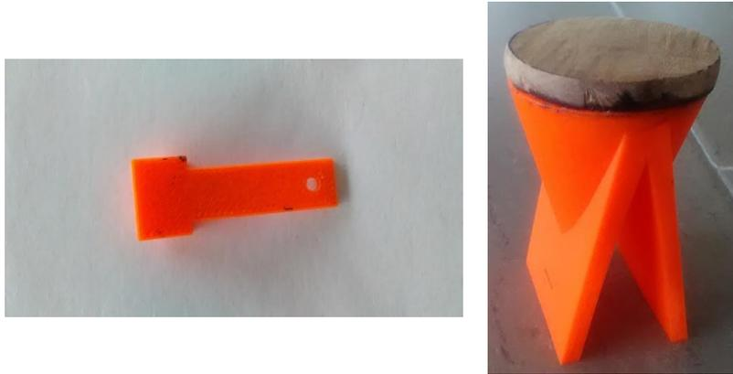
Figure 6 The wing connector (right) and motor mount (left) produced by Zortrax M200 3D printer.
