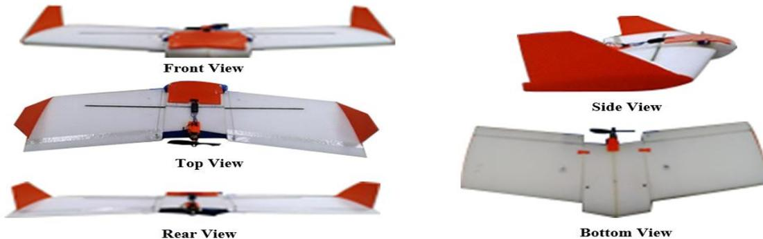
Figure 7 Final assembly of Neo-Ptero  $\mu$ -UAV model
