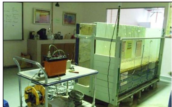
Figure 2: Model 2 with Soil Moisture Probe – Undrained condition
