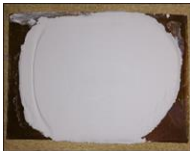
Figure 2. Fabricated barium titanate piezoelectric sensors with a copper substrate at the dimension of 0.1 mm × 35 mm × 50 mm.
