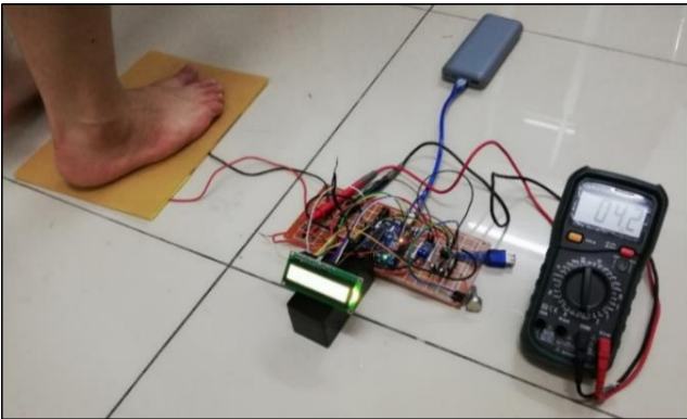
Figure 6. Output voltage measurement setup for footstep power generator.
