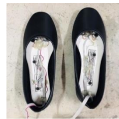
Figure 3. Vibrating Insole Prototype in Footwear
